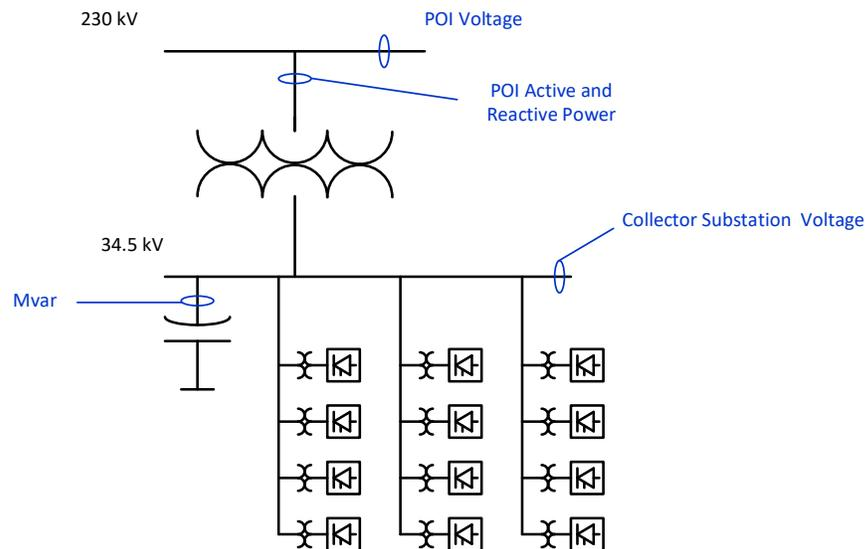
**Figure 11.---Test measurement points**
