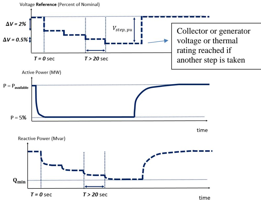
**Figure 44.--- Generic Test Recordings for the Lower Active Power Reactive Capability Test**
