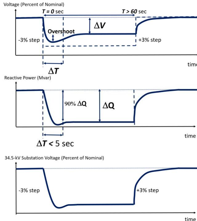
Figure 22.--- Generic Test Recordings for the Voltage Step Test
