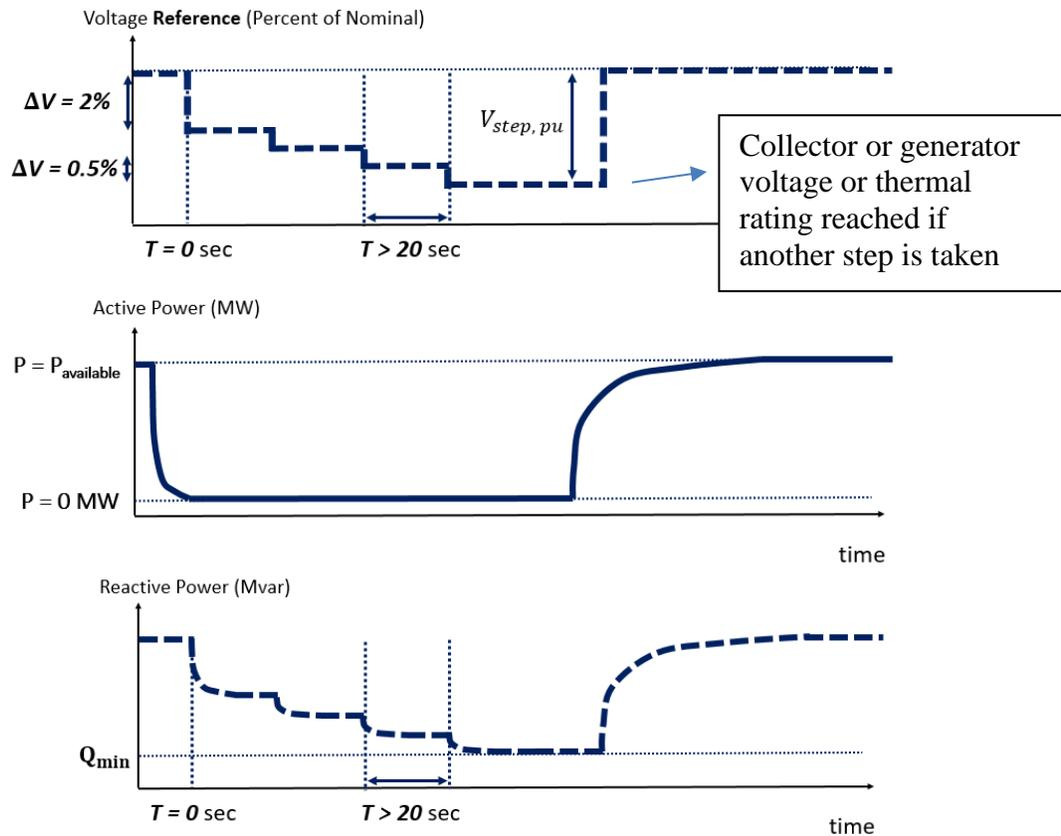
**Figure 33.--- Generic Test Recordings for the Lower Active Power Reactive Capability Test**
