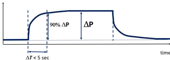
**Figure 66. Generic Test Recordings for the Under-Frequency Step Test**
