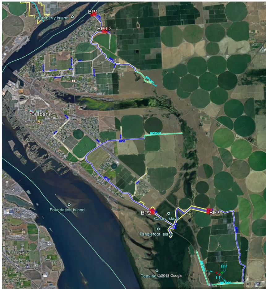
Figure F-6. Location of pumps and wasteways for Blocks 2 & 3. BP1 and BP1WW provide the feed and waste for Block 2. BP2, BP2WW, BP3, and BP3WW provide the feed and waste for Block 3. Image courtesy of John Anderson, USBR.
