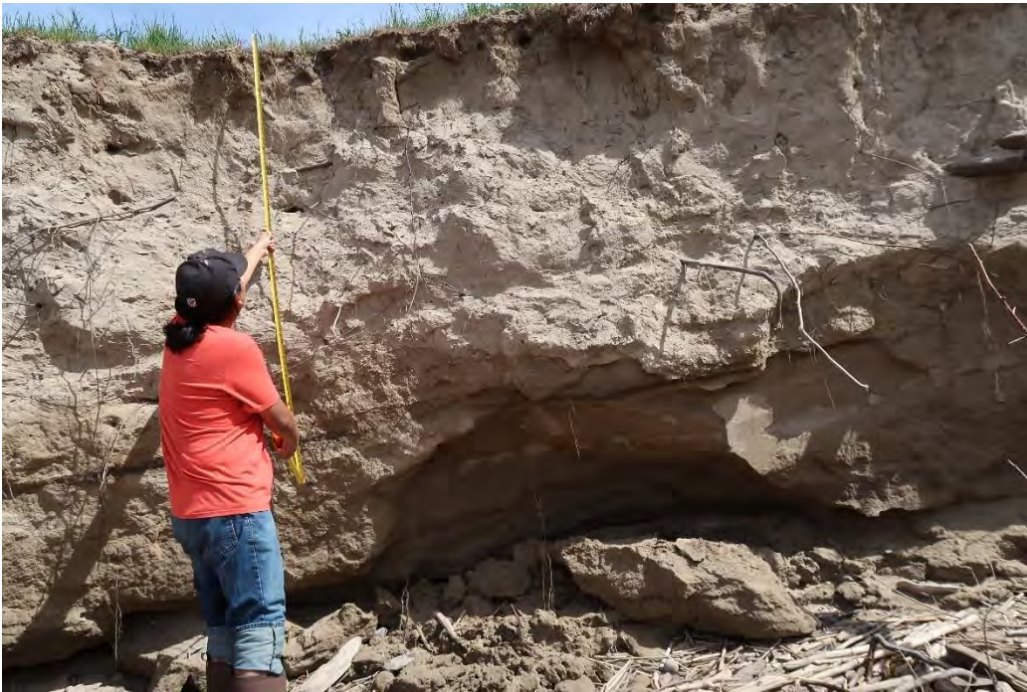
Figure F-5. Site monitoring at 45WT10 by the Nez Perce Tribe at Little Goose in FY 2022. The cutbank, after remaining relatively stable for approximately a decade, has now been undermined by fluctuating water levels.
