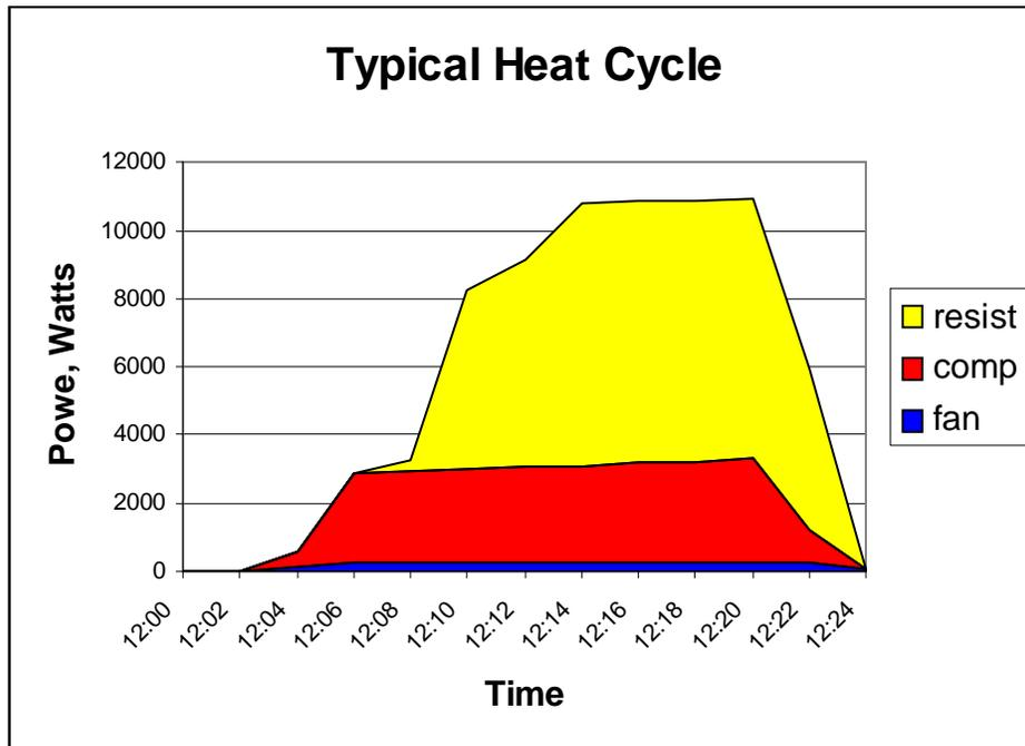
The COP of this system with the discharge sensor in play was very poor (around 1, or close to the COP of electric resistance alone). When the discharge sensor was disabled, the house stayed at setpoint and the COP improved to what is expected for a heat pump.
