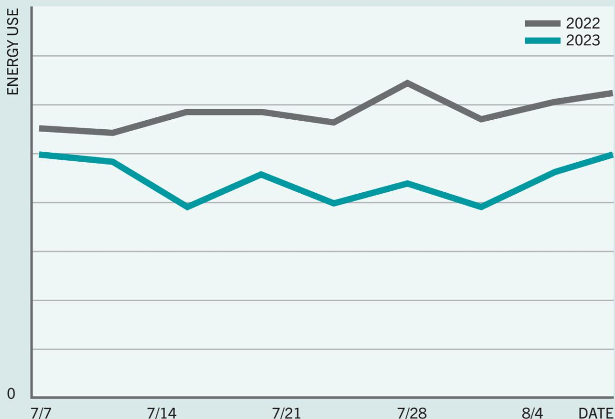
Fruitsmart operates a fruit processing plant and a cold storage in Prosser, WA. In 2023, they implemented several projects to improve refrigeration energy efficiency. The installed measures produced a substantial drop in year-over-year energy—more than originally estimated.
