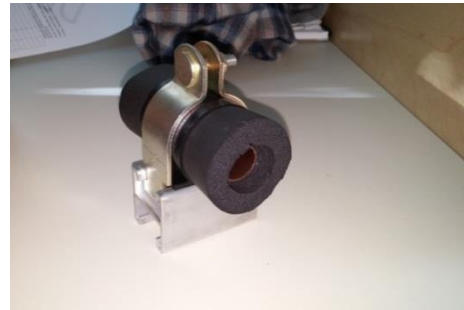
Figure 8: Recommended Configuration for Full Pipe Insulation
