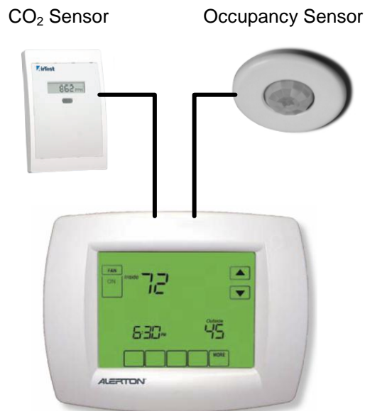
Temperature Sensor and Schedule/Setpoint Adjustment
