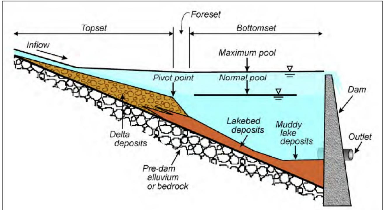
**Figure 3.3-2. Idealized Sediment Profile within a Dam-controlled Reservoir.**
