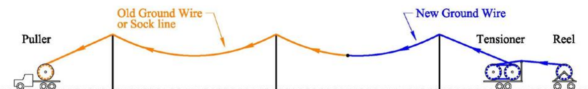
Figure 3. Typical Stringing Operation
